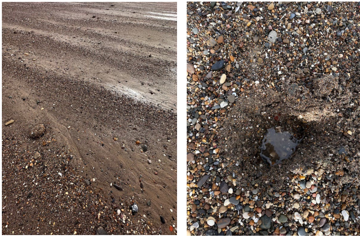
Plate 3-6 Example of the sand with overlying shingle zone found in Landfall 8 & 9 and representative dig-over
