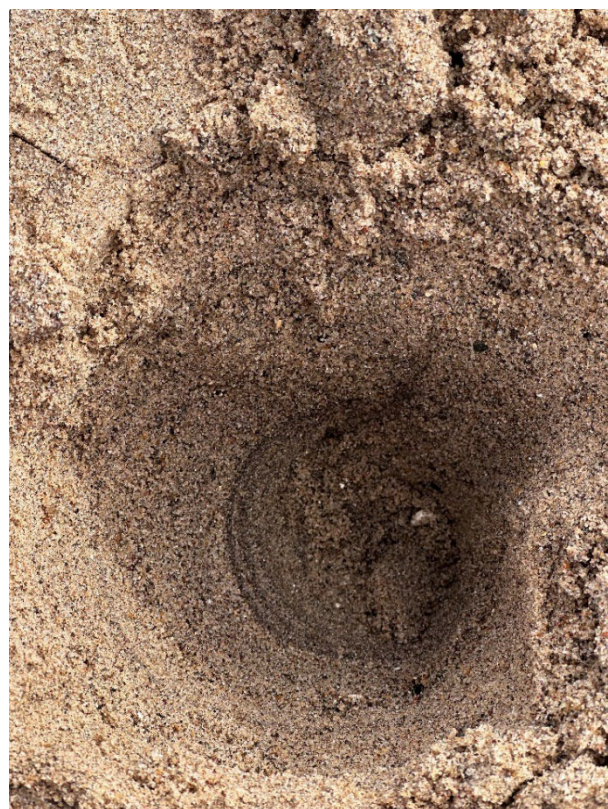
Plate 3-4 Example of the medium / coarse sand zone found in Landfall 8 & 9 and representative dig-over
