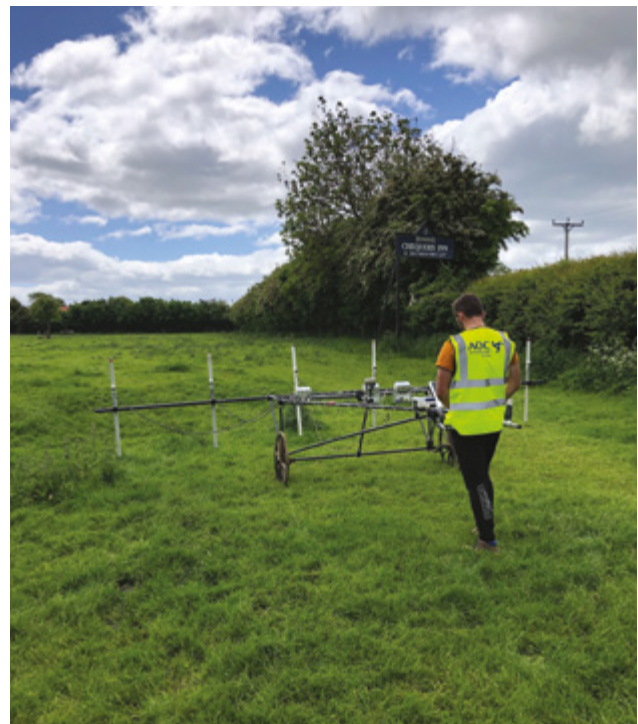
A gradiometer fitted to a hand-pushed cart used during archaeological surveys.
